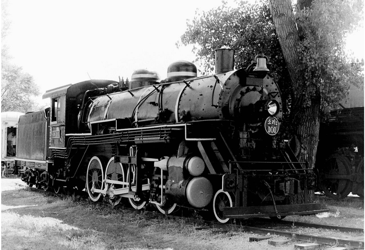
A U.S. Army 101 a 2-8-0 locomotive manufactured in 1916, issued in World War One.
